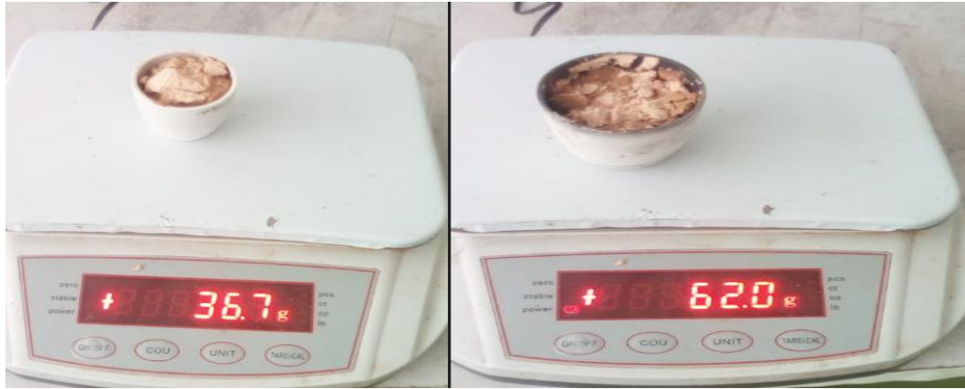
Picture 2 Measuring of the moisture content of the spent kiselghur after perpartion of the adsorbent
