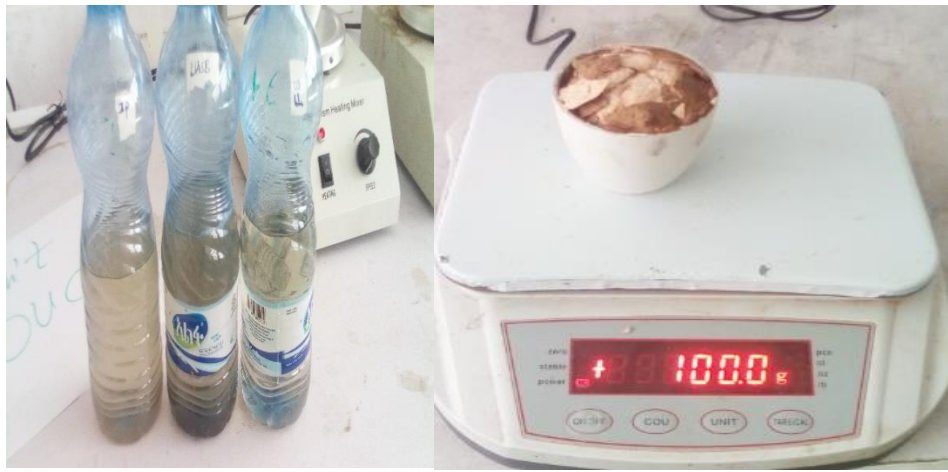
Picture 1.The raw sample of the waste water and spent kiselghur with the measuring of the moisture content
