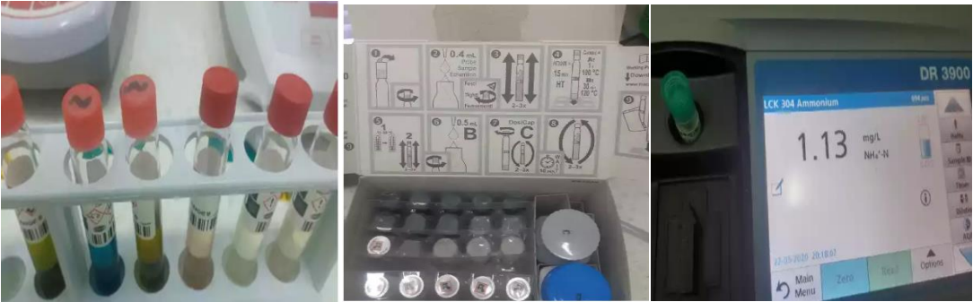
Picture 11 The final experiment of the phosphate, nitrate, COD, BOD in the habesha bewry factory
