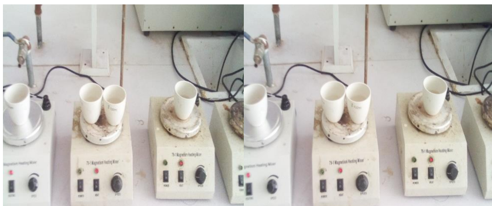
Picture 9 Total dissolved solids measuring process
