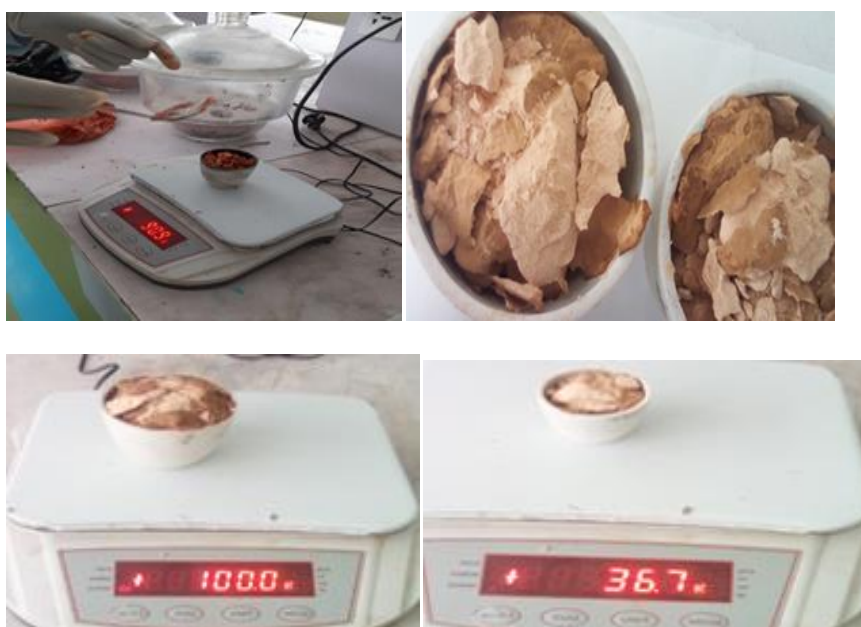
Figure 3. 2 the moisture content of sample prepared kiselguhr and preparation of adsorbent and the instrument.
