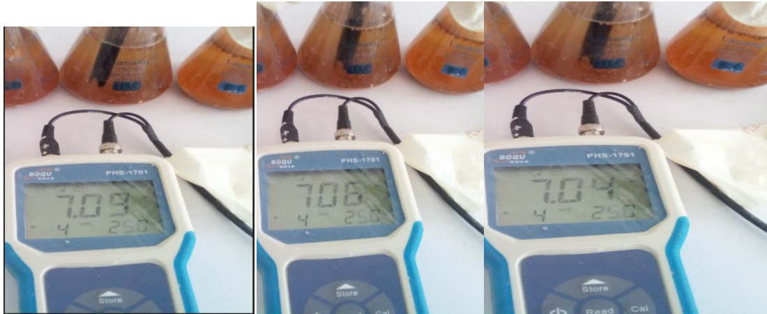
The UASB PH result at atm. temperature with 63 p.size,48,60,72,hr respectively with order
