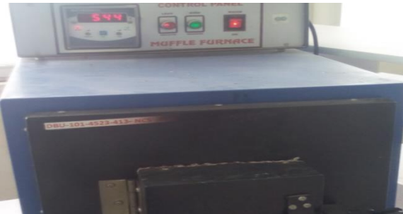
Muffle furnace for ash content measurement
