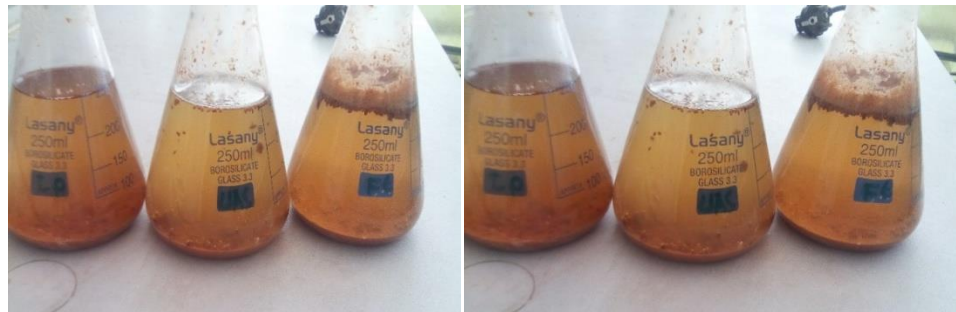
Picture 7 The final experiment sample after extra reaptation process with 60hr, and 72hr.time investigation and particle size of 63 micro meter.
