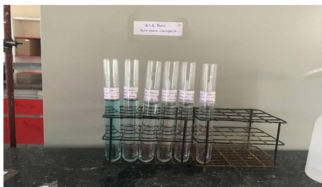
MB dye degradation using CNCs/Ag@ZnO (1:1) BNC
